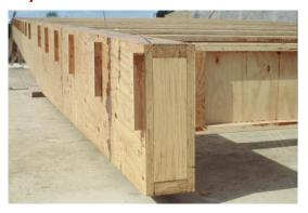
Structural plywood to AS/NZS 2269.0 can be simply nailed to timber or LVL flanges to form structurally efficient but lightweight plywood webbed C or box beams. Plywood webbed beams can provide economical lintels of roof beams in residential constructions, or rafters, columns and purlins in industrial type buildings.
